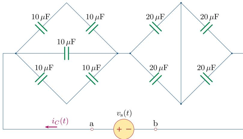
b) Calculate the equivalent capacitance  $C_{\text{eq}}$  at the terminals a–b. (2 points)
