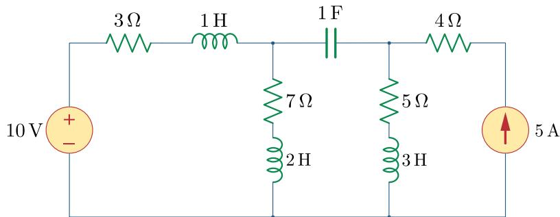
d) Calculate the total energy  $w_{\text{tot}}$  stored in the capacitor and the three inductors. (4 points)
