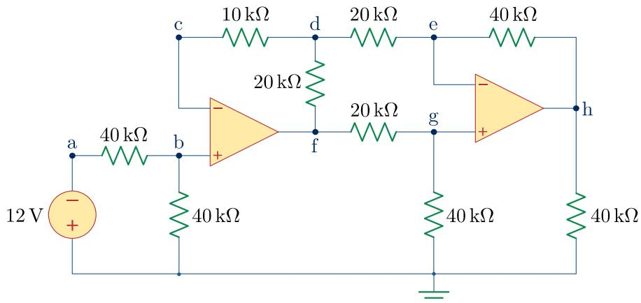
c) Calculate the nodal voltages a – h in the circuit, by assuming both op amps to be ideal. (5 points)
