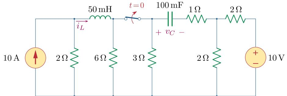
The switch has been closed for a long time. At  $t = 0$  the switch opens.
