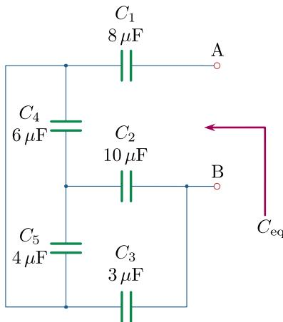
b) Calculate the equivalent capacitance  $C_{eq}$  at the terminal A–B. (2 points)
