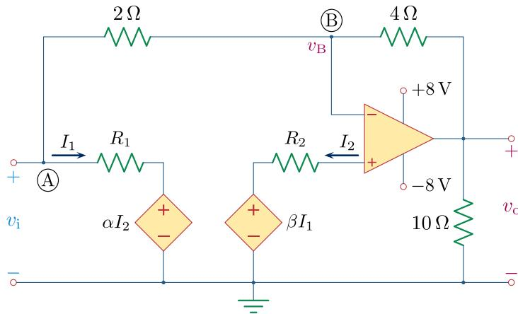
a) Calculate the ratio of voltage at node B over the input voltage ( $v_B/v_i$ ). State your answer in terms of  $R_1$ ,  $R_2$ ,  $\alpha$  and  $\beta$ . (3 points)
