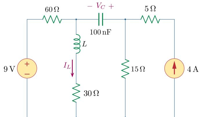
c) Calculate the current  $I_L$  through the inductor and the voltage  $V_C$  across the capacitor. (3 points)
