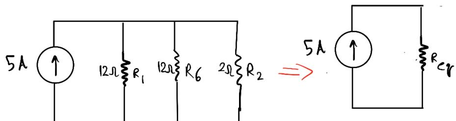
Calculating the equivalent resistor  $Req$ :
