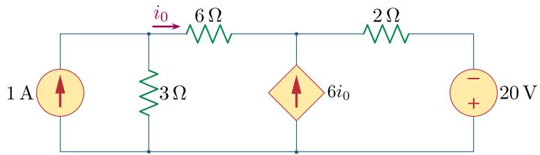
b) Calculate current  $i_0$  using mesh analysis. (4 points)
