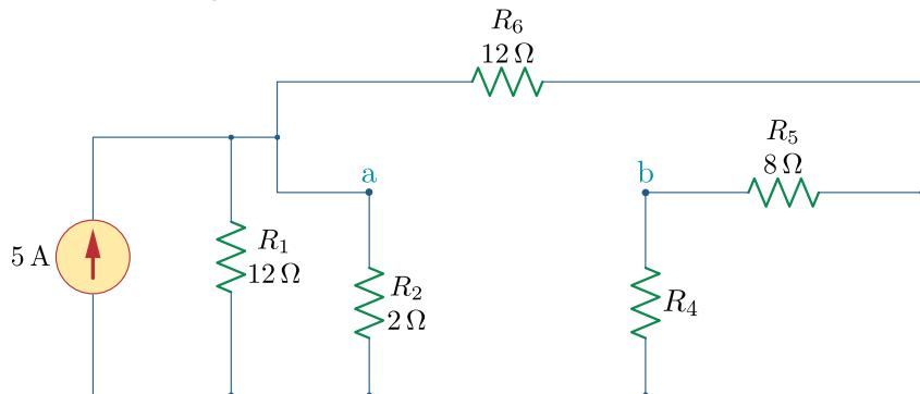
a) Determine the power delivered by the 5A current source. (3 points)
