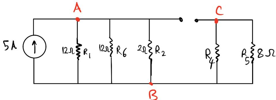
Clearly,  $R_4$  and  $R_5$  are not part of the circuit and we are left with 3 resistances in parallel. With this in mind, the remainder of the solution is straightforward.
