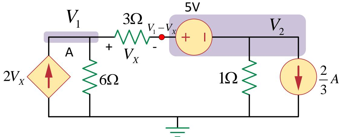
$$\text{KCL (A): } \frac{V_1}{6} + \frac{V_x}{3} - 2V_x = 0$$
