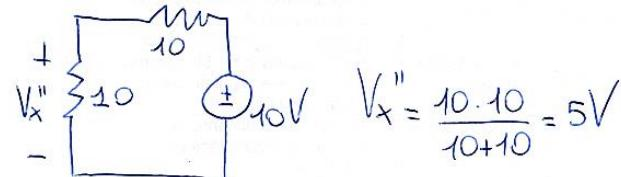
The final result is obtained by adding the two partial results:
