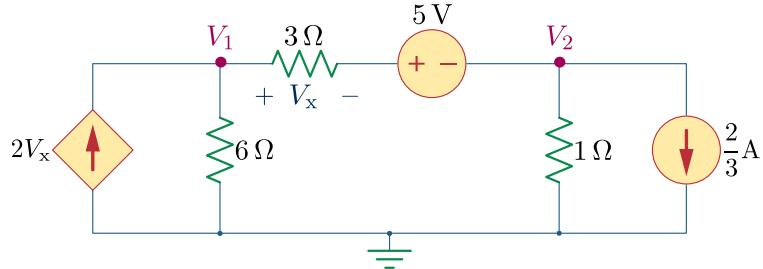
a) Calculate voltages  $V_1$  and  $V_2$  using the nodal analysis. (6 points)
