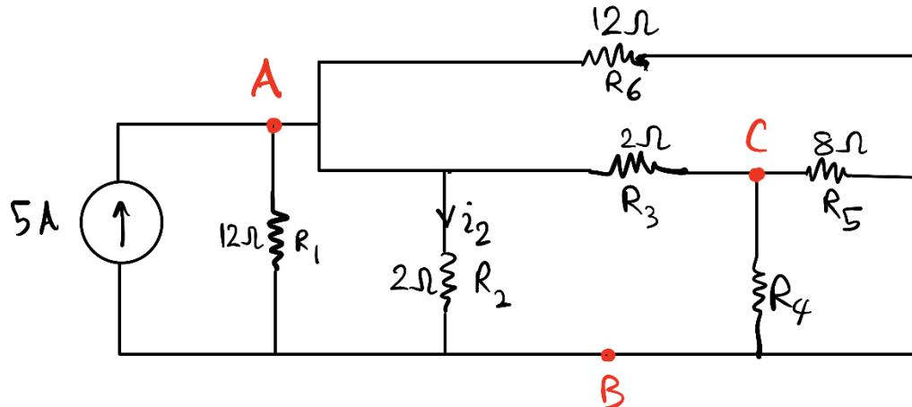
Examining those nodes shows that the new circuit has important similarities with the previous: we have the same 3 resistances in parallel and a new group consisting of  $R_3 + (R_4 \parallel R_5)$  which is also in parallel with the previous group (see the new schematic below).
