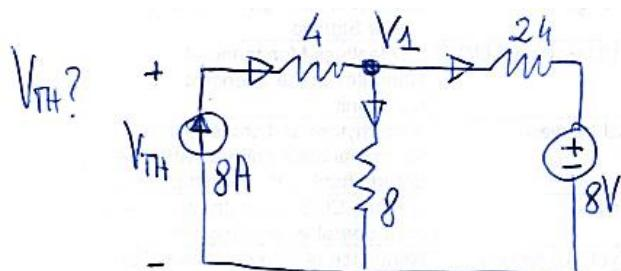
For calculating the Thévenin voltage V<sub>Th</sub> we apply KCL at the node 1 → the relevant equations are given below
