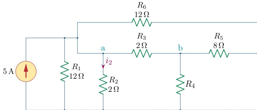
b) Determine the value of the resistance  $R_4$  by knowing that the current flowing through  $R_2 = 2\Omega$  is now  $i_2 = 3A$ . (4 points)
