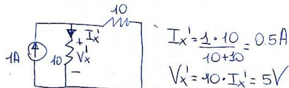
while turning off the 1A current source results in the circuit:
