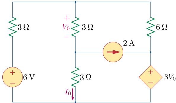
a) Label the nodes in the network and assemble the corresponding system of equations for nodal analysis, when applied to this circuit – **do not solve the system of linear equations yet!** (4 points)
