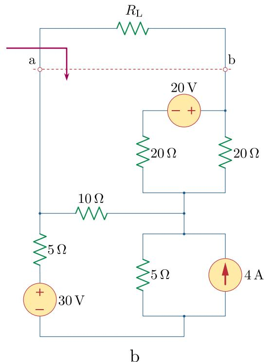
a) Find the Norton equivalent at the terminals a–b of the circuit. (5 points)
