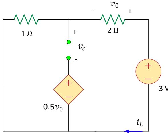
3 volts is across the 2 and 1 ohm resistors, therefore  $v_0 = 2 V$  and  $i_L = -\frac{3}{3} = -1 A$
