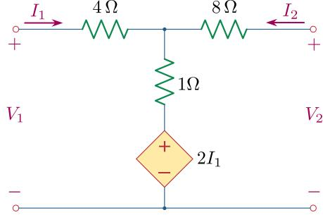
a) Calculate the  $Z$ -parameters  $z_{11}$ ,  $z_{12}$ ,  $z_{21}$  and  $z_{22}$ . (5 points)
