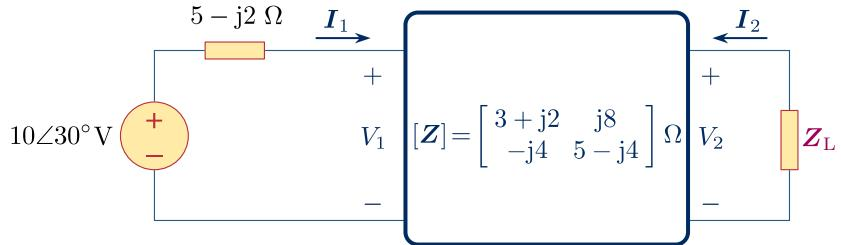
b) Redraw the circuit with all independent sources pasivised (set to zero) and the load replaced by a current source with the value  $I_{\text{test}}$ . (1 point)
