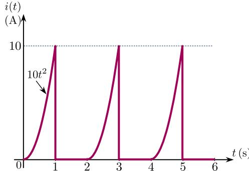
a) Obtain the rms current  $I_{\text{rms}}$  of this current. (3 points)
