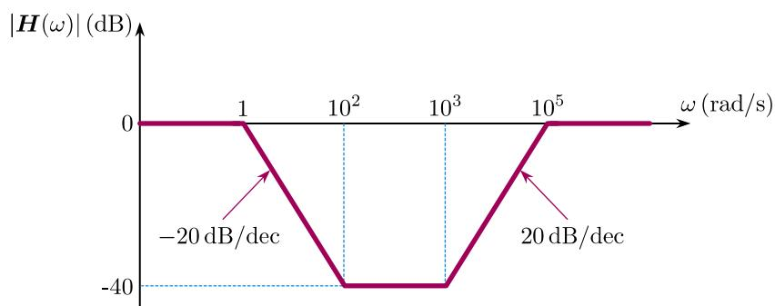
b) Find the corresponding transfer function  $H(\omega)$ . (5 points)
