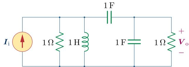
a) Find the transfer function  $H(\omega) = \frac{V_o}{I_i}$ . (5 points)
