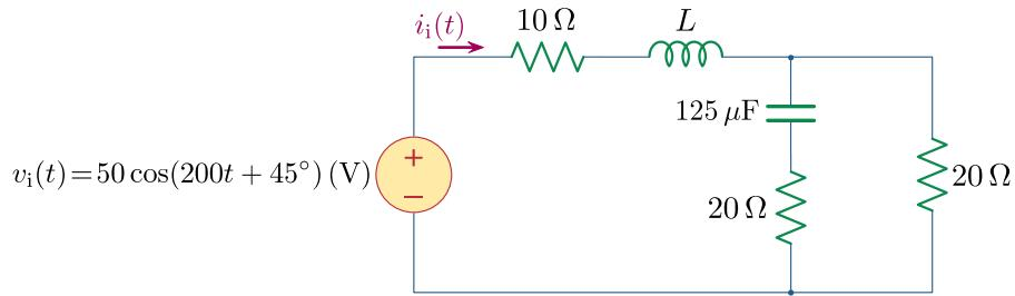
b) Calculate the value of the inductance  $L$  such that to ensure that the phasor-domain input current  $\mathbf{I}_i$  is in phase with the phasor-domain input voltage  $\mathbf{V}_i$  (or, in time-domain,  $i_i(t)$  does not lead or lag  $v_i(t)$ ). (4 points)
