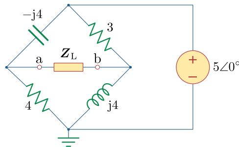
b) Calculate the Thévenin voltage  $\mathbf{V}_{\text{Th}}$  at the terminals a – b. (3 points)
