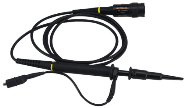
Probe (note: make sure you check attenuation (1x or 10x) on both probe and oscilloscope channel settings)
