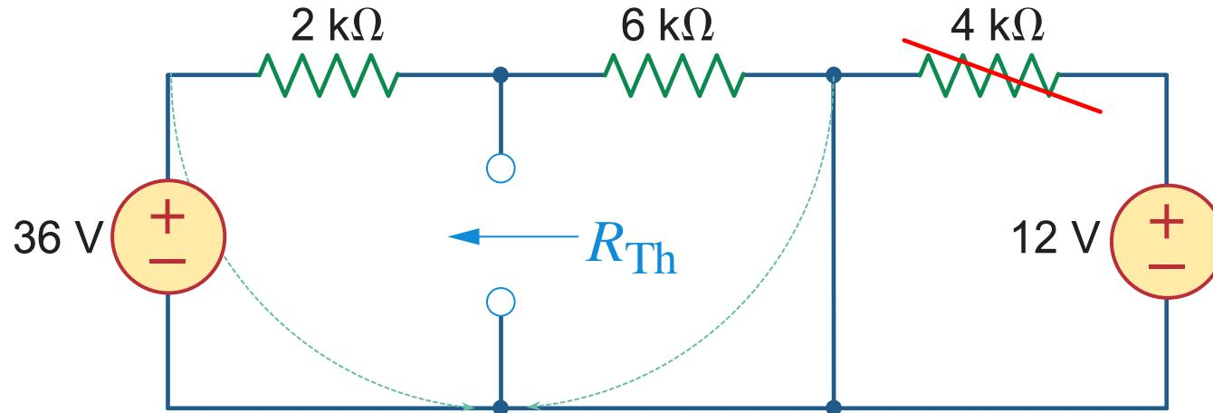
$$R_{Th} = \frac{(2k)(6k)}{2k + 6k} = \frac{3}{2} \text{ k}\Omega \quad \longrightarrow \quad \tau = R_{Th}C = \left(\frac{3}{2}\right)(10^3)(100)(10^{-6}) = 0.15 \text{ s}$$
