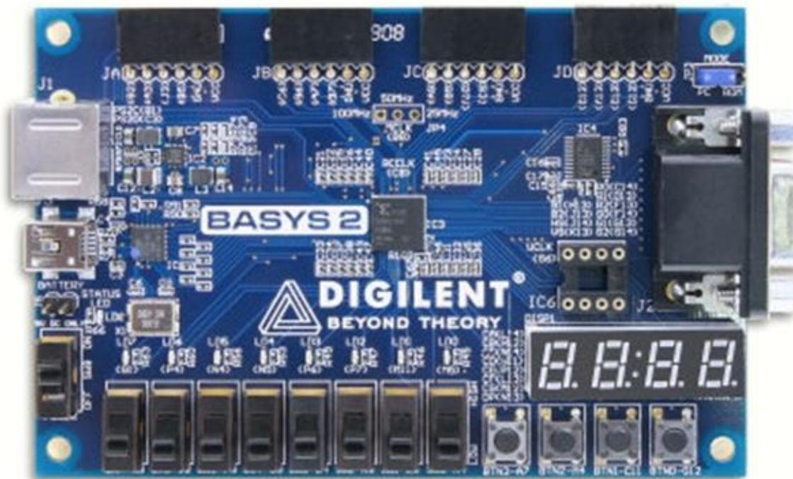
FPGA contains components that are connected by switches controlled by RAM memory
